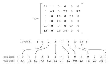
Fig. 1. The CSR sparse matrix storage format.
