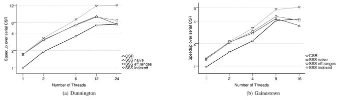
Fig. 9. Symmetric SpM×V speedup with different local vectors reduction methods. The significant memory traffic incurred by the naive and the effective ranges technique as the number of threads increases eliminates any benefit from the gain of the symmetric storage.
