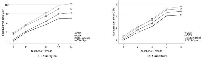
Fig. 11. Symmetric SpM×V speedup with the CSX-Sym format. All symmetric formats use the optimized local vector indexing method..
