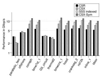
Fig. 12. Per-matrix performance for the CSX-Sym format at 16 threads in Gainestown. CSX-Sym's performance in more regular matrices surpasses 10 Gflop/s, while staying close to baseline CSR performance in less regular ones.
