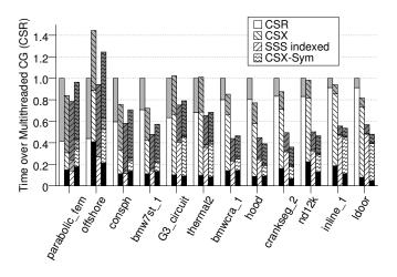
Fig. 14. CG execution time breakdown using 24 threads in Dunnington at the RCM reordered matrices after 2048 iterations. [Execution time breakdown legend – white: SpM×V, light gray: SpM×V reduction, dark gray: vector operations, black: CSX/CSX-Sym preprocessing.]
