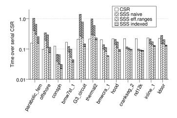
Fig. 10. Symmetric SpM×V execution time breakdown at 24 threads in Dunnington. The reduction overhead (shaded regions) is considerably reduced with the use of local vector indexing.
