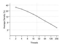
Fig. 4. The density of the effective regions of local vectors. Local vectors become more sparse as the thread count increases, reaching a 2.7% density at 256 threads. The vertical line marks the density at the 24 threads of the Dunnington system.
