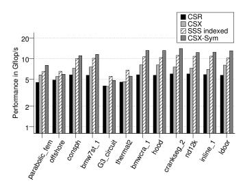
Fig. 13. Per-matrix performance on reordered symmetric matrices (Gainestown, 16 threads).
