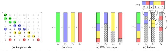
Fig. 3. Local vector methods for the reduction phase of the symmetric SpM×V kernel. An example implementation of symmetric SpM×V with p = 4 threads. The naive method (b) uses simply four local buffers that reduces later to the final output vector. The effective ranges method (c) uses p - 1 local vectors writing only the possibly conflicting regions. The indexing scheme proposed 3d uses p - 1 local vectors and an indexing structure that points only to the really conflicting elements.
