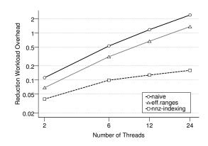
Fig. 5. The workload overhead of the reduction phase (over the serial SSS implementation) for the three local vectors methods considered. The overhead of the indexing scheme proposed tends to stabilize as the thread count increases.
